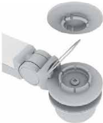
Step 1: Lift metal ring and slide end of LIGEO™ SLC into connector hub.
